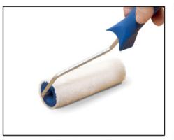
2. Apply the wallpaper adhesive to the back of the fresco with a paint-roller and cover the entire surface with a polyethylene film.
